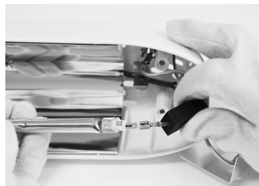
6. CONNECT THE MALE FASTONS TO THE NEW BULB TO THOSE OF THE TWO CORDS. COVER THEM WITH THE CAPS AND REPOSITION THE BULB IN THE SEAT OF THE TWO SPRING CLIP. DO NOT TOUCH THE BULB WITH YOUR BARE HANDS. REASSEMBLE THE DEVICE BY PERFORMING THE ABOVE TASKS IN REVERSE ORDER.
