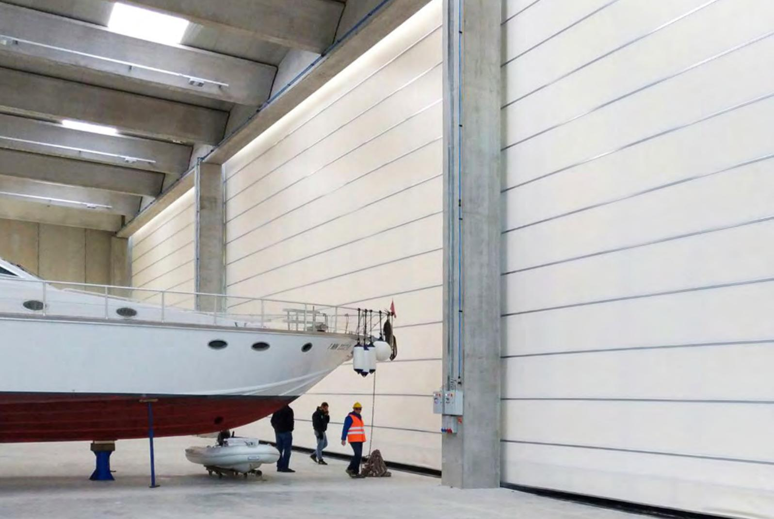
The **MEGAPACK®** fold-up door is the technological evolution of heavy industrial doors used to close big gates, now inappropriate and obsolete for today's industrial needs.
