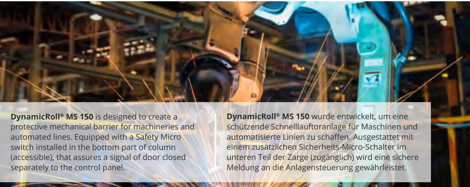
**DynamicRoll® MS 150** is designed to create a protective mechanical barrier for machineries and automated lines. Equipped with a Safety Micro switch installed in the bottom part of column (accessible), that assures a signal of door closed separately to the control panel.
