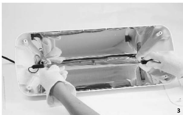
3. RELEASE THE BULB FROM THE CLAMPS.
